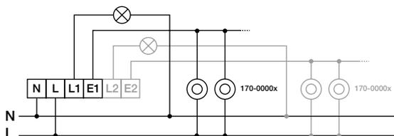
Connect the contacts of the traditional push button to the L terminal and E1 terminal of the smart switch. Use terminal E2 to extend the second channel of the smart switch (only applies to the 410-002x0) with traditional push buttons.
